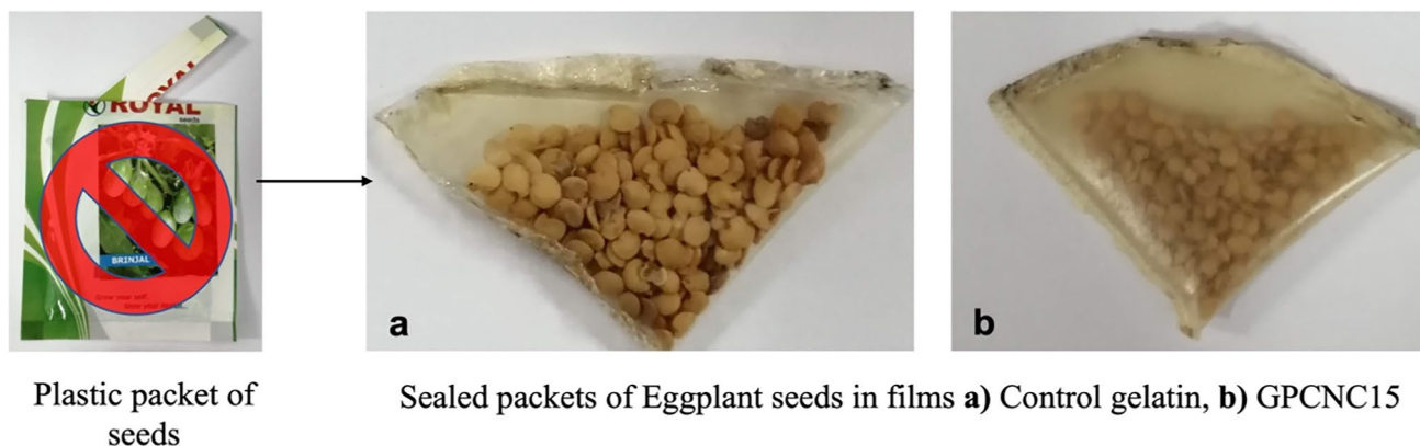
Fig. 11 Packaging performance of nanocomposite films a control gelatin; b GPCNC15
