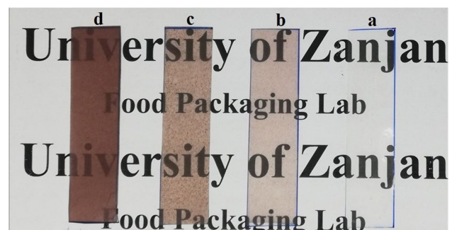
Fig. 1 Visual properties of the starch (a) and starch/ Fe 3 O 4 /TiO 2 nanocomposite films with different Fe 3 O 4 /TiO 2 content 3% (b), 5% (c), 10% (d) with backlight
