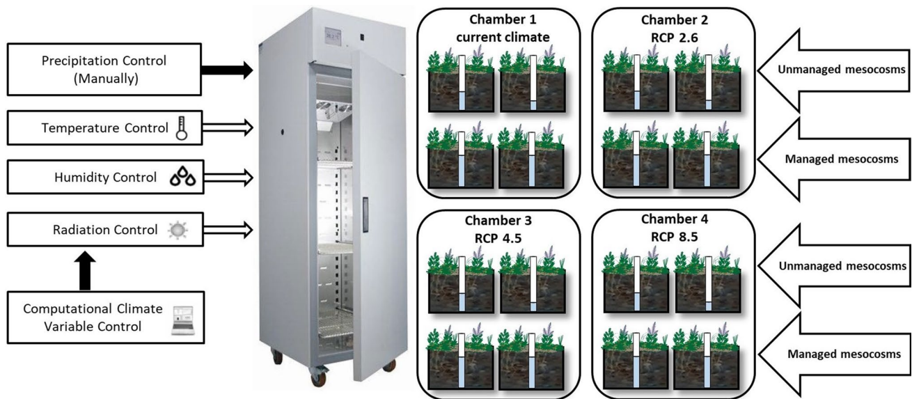
Fig. 1 Design of mesocosm experiment in climate control chambers simulating the current and future representative concentration pathway (RCP) climate scenarios and water level management for peatlands during 2018–2020. During the first year of the experiment, all four peatland mesocosms were subject to water level management
