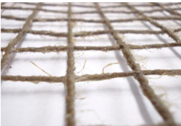
Fig. 9 The grid of hemp fibers: this was embedded into a 15-mm lime (pozzolanic) coating (Menna et al. 2015)
