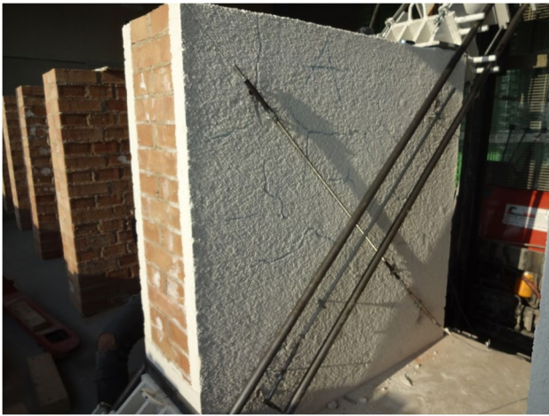
Fig. 5 FRCM reinforcement using lightweight mortar mixes: to increase the thermal resistance of the wall, the thickness of the coating needs to be enlarged (typically 100 mm). The weight density of the mortar, used for the coating, can be reduced up to 800 \text{ kg/m}^3 without significantly affecting the strengthening effect of the FRCM (Borri et al. 2016)
