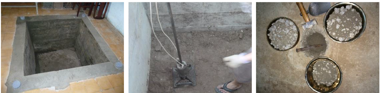
Fig. 3 Reinforced concrete hole, hand compactor, and measure the degree of compaction
