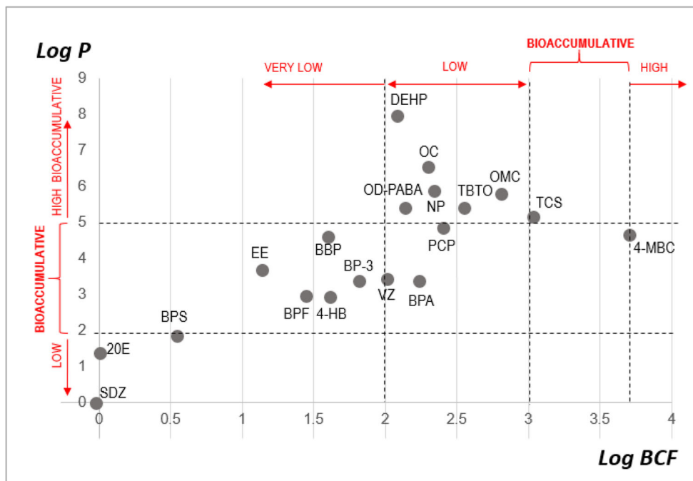
Fig. 4 Bioaccumulation potential. Log bioconcentration factor (BCF, defined as the ratio of the amount of chemical in an aquatic organism to the amount of chemical in the water under conditions of equilibrium) versus \text{miLog}P , where P is the octanol-water partition coefficient. Both indicators have been calculated by Molinspiration ( https://www.molinspiration.com )
