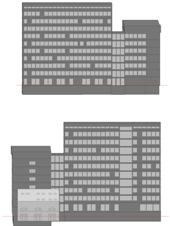
Fig. 2 View of facades (west facade above, east below)—model of existing building FBSHEE
