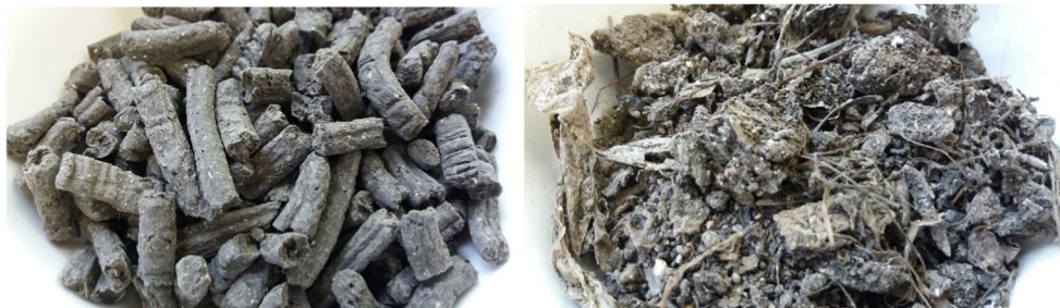
Fig. 1 Photographs of feedstock materials. Sewage sludge (SS) pellets (left) and composted organic fines (OF) from municipal solid waste (right)
