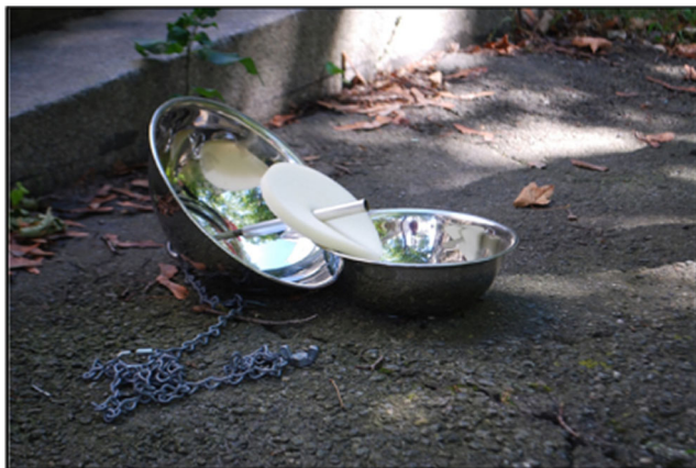
Fig. 3 Passive monitoring apparatus for PCBs in ambient air
