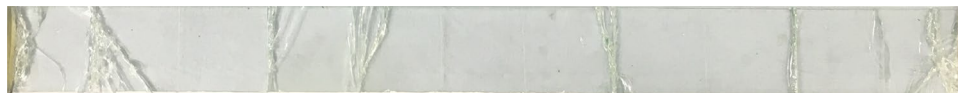
Fig. 18 Post-experiment crack pattern for pre-scored specimen with 0.76 mm interlayer tested at 10 m/s (specimen no.19)
