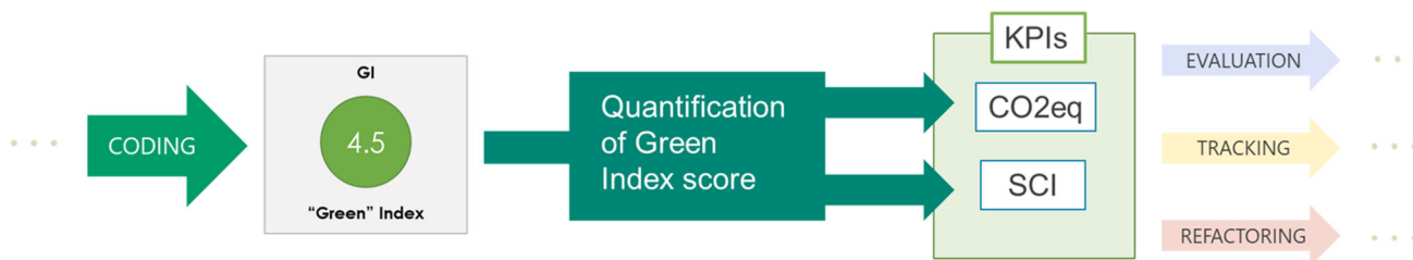
Fig. 4 Green coding pipeline: static analysis of code, Green index quantification, emissions evaluation and code optimization
