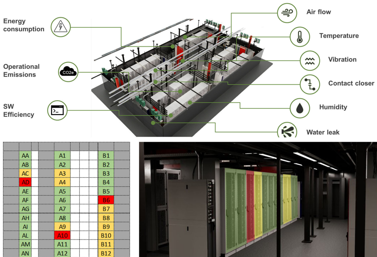
Fig. 9 Data center digital twin environmental monitoring
