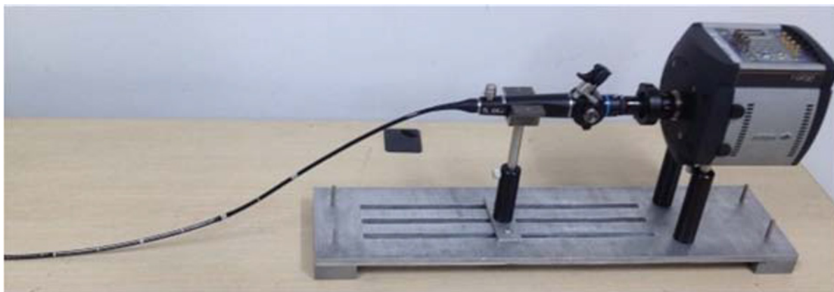
Endoscopic Cerenkov luminescence imaging system
