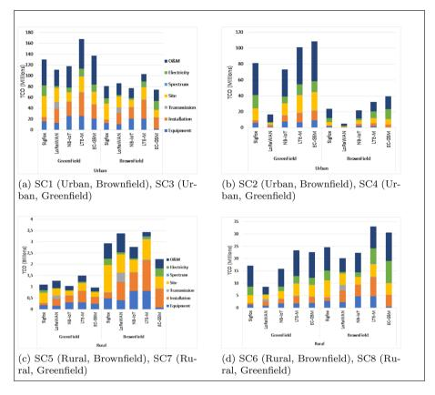
Fig. 6 TCO of different deployment options
