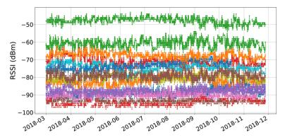
Fig. 2 A typical sequence of RSSI measurements showing how one AP is heard from all its neighbours in the 2.4 GHz
