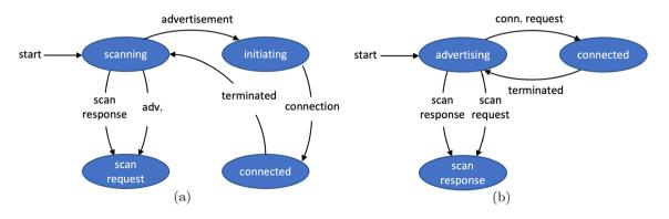
Fig. 1 BLE connection process: a Master or central b Slave or peripheral
