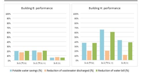
Fig. 7 Performance results for the studied Building B and Building H
