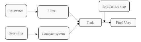
Fig. 1 Configuration of hybrid systems
