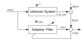
Figure 1 Adaptive system identification.
