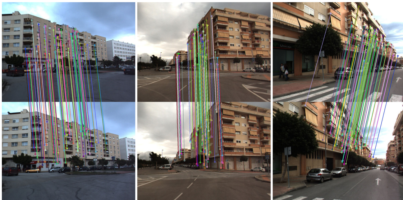
Fig. 7 Example image pairs and inliers of homographies estimated by the proposed 1SIFT solver from the Malaga dataset. Outliers are not visualized. Only 100 randomly selected inliers are drawn (Color figure online)
