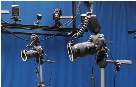
Fig. 15 Acquisition setup consisting of a pair of cameras fitted with external flashes mounted on each camera lens
