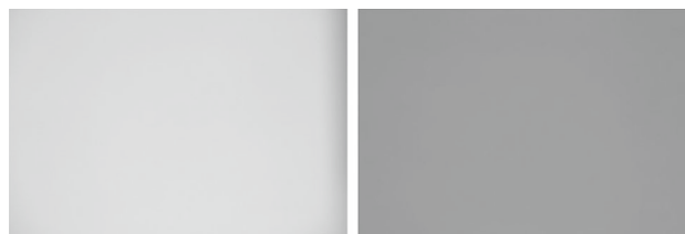
Fig. 4 Calibration images of a uniform plane used for deriving average brightness focused at infinity (left) and at a focus setting (right). Besides the focus distance, all camera parameters and lighting conditions remain constant in both images. The observed change in brightness is therefore attributed to the pupil ratio. Images are white balanced and brightened for visualisation
