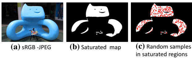
Fig. 5 This figure shows an example of saturation encoding. a The original sRGB-JPEG image. b The saturation map, which is identified from (a) . c Spatial samples locations (red dots) that are randomly sampled in these saturated regions (Color figure online)
