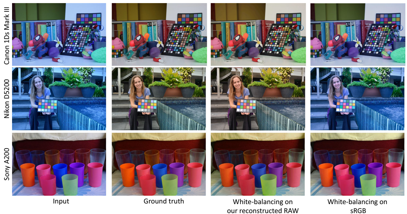
Fig. 11 This figure shows examples for correcting white balance for different cameras: a Canon 1Ds Mark III, a Nikon D5200, and a Sony \alpha 57. The first column is the input images captured under the wrong white-balance settings; the second column shows the ground truth
