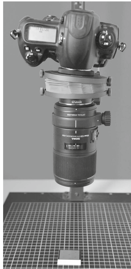
Fig. 18 The experimental setup used to obtain the results in Table 2. A Sigma 150 mm F2.8 macro lens and a Nikon D3 camera were attached to the Novoflex Balpro T/S bellows. The image also shows the calibration object
