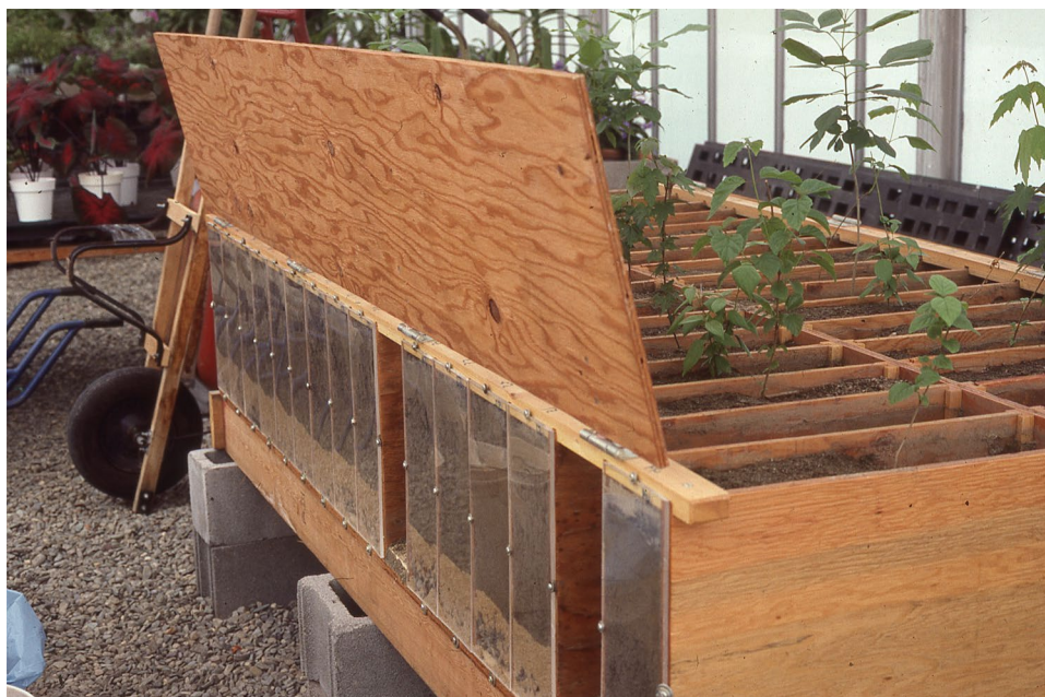
Fig. 1 The experimental planting boxes with nutrient gradients after several plants reached the plexiglass-covered end wall and were harvested
