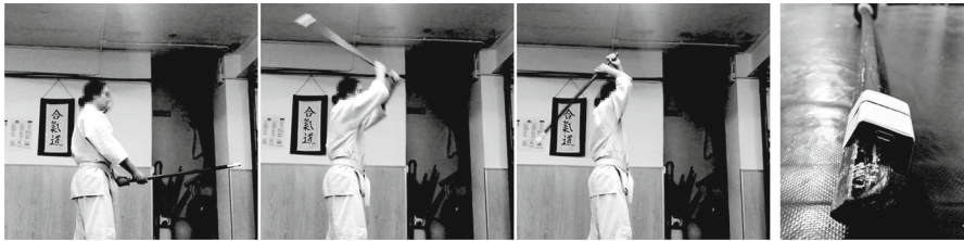
Fig. 2 Three left images represent one straight blade swing ( bokken shomenuchi ) sequence performed by an Aikidō practitioner (who authorised the recording and publication of the images). The rightmost image shows the experimental setup comprising an AX3 accelerometer tightly attached to the tip of one of these wooden Japanese swords
