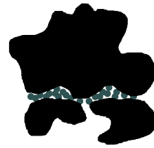
The smallest particles form a “glue” or “cement” for the bigger particles
