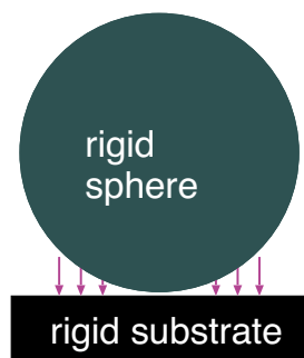
Fig. 8 If the solids are assumed rigid the sphere will be in contact with the flat in a single point. The two objects attract each other by a force field which is large only close to the contact point
