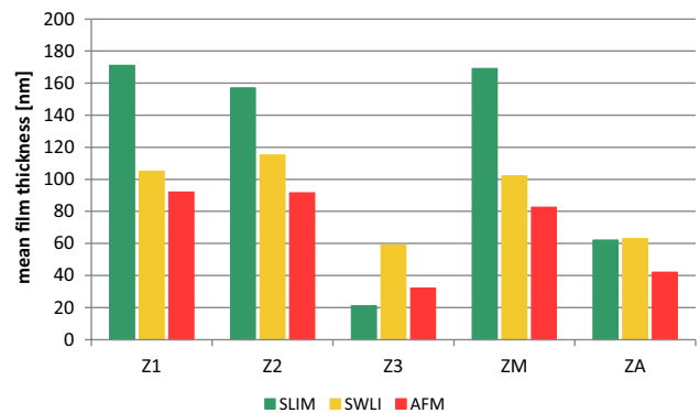
Fig. 13 Comparison of mean tribofilm thickness results of ZDDPs using three measurement methods
