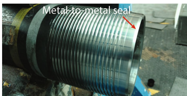
Fig. 1 Male or “pin” member of a premium casing connection assembly. The pin is connected to a female or “box” member by the thread. At the final moment of assembly, the metal-to-metal seal engages ensuring a gas tight connection
