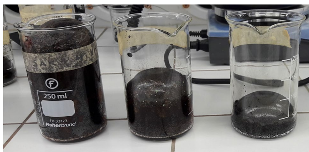
Fig. 2 Photograph of foams prepared with different nickel amounts. Highest 4 m% of nickel on the left, middle 2 m% of nickel and on the right 1 m% of nickel
