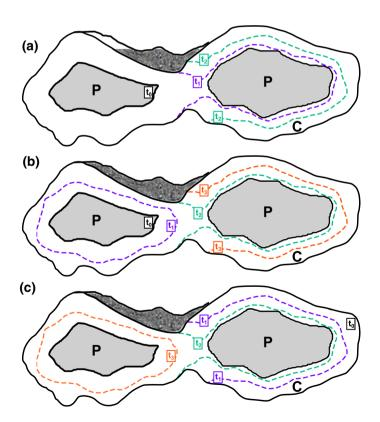
**Fig. 1** Sketch illustrating the different methods of back-stripping  $(\mathbf{a}, \mathbf{b})$  and the simulated precipitation  $(\mathbf{c})$ , for two amygdales partially filled by calcite (C), and including a central pore filled by air (P). The air-filled paleo-porosity  $(t_0)$  is indicated by a solid black line
