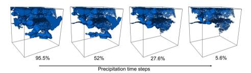
**Fig. 8** Temporal evolution of connected porosity  $(\phi_c)$  in blue with calcite precipitation along the *X* direction for four steps of the simulated precipitation. The percentages indicate the volume of surface connected porosity against total porosity  $(\phi_c/\phi_{tot})$ , cfr. to Fig. 6c). The remaining space of the sample is filled by the basaltic matrix, that is not represented here. Vertical side is 13.6 mm long
