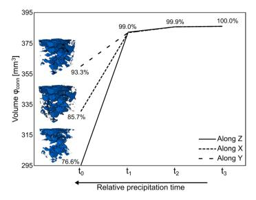
**Fig. 4** The graph shows calcite precipitation through relative time.  $t_n \phi_c$  is reported (in mm<sup>3</sup> and as percentage connectivity ( $\phi_c/\phi_{tot}$ ) against time of precipitation for each direction. The precipitation time, right to left ( $t_3$  to  $t_0$ ), is represented by different stages of morphological dilation, from left to right. 3D renderings for each direction are represented in blue models
