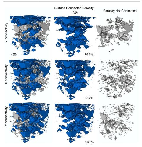
**Fig. 3** 3D renderings showing the connected porosity  $(t_n\phi_c)$ , in blue), and the non-connected porosity (white) for different direction of flow at current time  $t_0$ . The percentage connectivity is also reported as  $t_0\phi_c/\phi_{\rm tot}$ . The remaining space, not figured in the images, is filled by the basaltic matrix and open (air-filled) porosity, which is represented by the air-filled fractures
