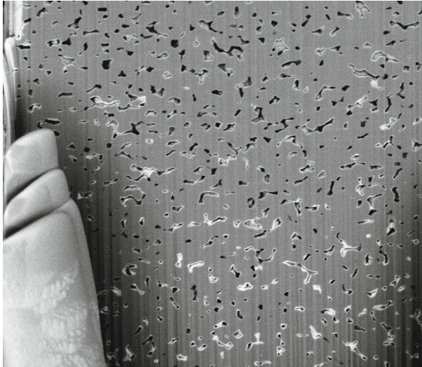
Fig. 6 Raw SEM image from face of milled column towards the end of the image collection sequence. Interference is noticeable with the intrusion of the remnants of the milled surface on the left of the image, as well as shadowing caused by the milled material
