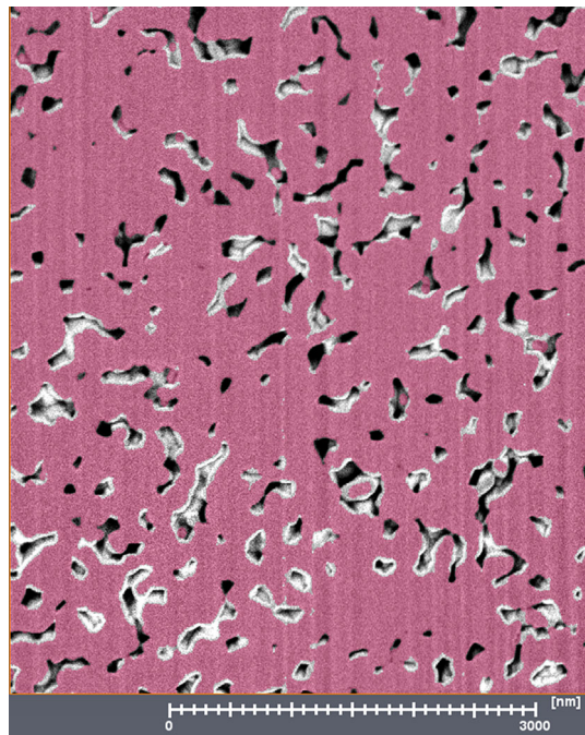
Fig. 8 Initial segmentation of pores from solid grains of ceramic B porous ceramic following filtering of image set overlaid on a x - y orthogonal slice of the collected volume. Pull-out section shows the small speckled regions within solid grains caused by image noise, as well as incorrectly “bridged” segmented regions around curved grain edges
