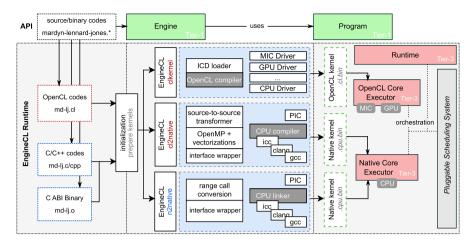
Fig. 1 EngineCL compilation-execution model showing the optimizations to enable different kernel origins via its new Core Executors functionality
