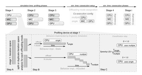
Fig. 2 Load balancing steps during the simulation: profiling, setup and co-execution phases
