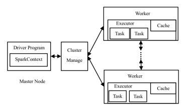
Fig. 1 Working model of Spark
