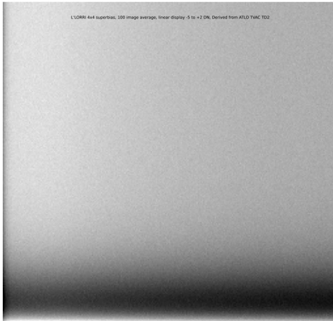
Fig. 19 Left: Mean of 100 4 × 4 bias images ( t_{exp} = 0 ms), which is called a superbias image. Right: Histogram of the superbias image. The positive tail is associated with the lowest rows of the image, and the negative tail is associated with the rows just above them
