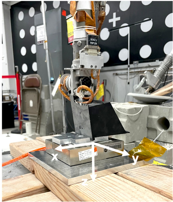
Fig. 28 Picture of the IDA scoop and multi-axis load cell in the testbed. Flat bottom of the IDA scoop is pressing on the multi-axis load cell setup at the Indentation and Elastic Properties location. Directions of the x -, y -, and z -axis forces are shown. Note the scoop tip to the right and the secondary blade on the bottom left. Note portion of calibration target (white circles on black background) against the wall behind the lander and the lander footpad to the right
