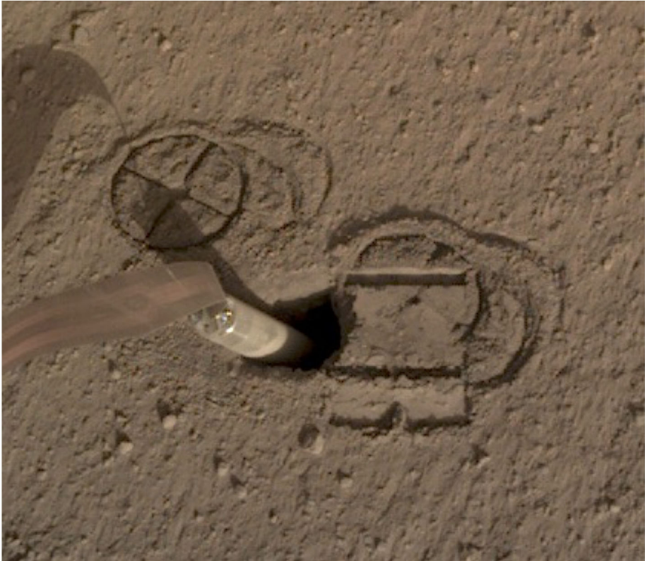
Fig. 11 Image of mole hole and surface after interactions with the HP 3 SSA feet and scoop. Circular cross patterns are imprints of the HP 3 SSA feet in the soil. Smooth, reflective rectangular surface is where the flat base of the scoop (7.1 cm wide) was pressed against the soil, causing a 5–10 mm indentation. Horizontal troughs near the top and bottom of the scoop imprint are where the front and back blades of the scoop (Fig. 4) penetrated into the soil
