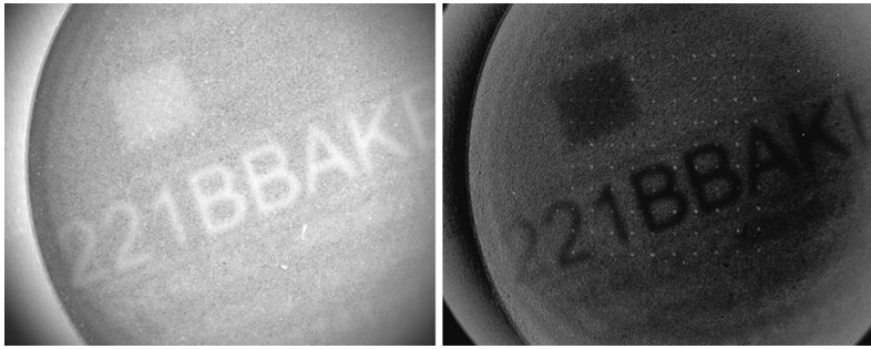
Fig. 11 Sol 59 ACI image of martian dust-coated polycarbonate spacesuit visor sample over geocache coin (left). Scale Reference: total target diameter is 25 mm; ACI images are full-frame images (1648 by 1200 pixels) acquired before and after the laser is fired, aligned, and subtracted. Bright spots in the right image represent differences in the target after the laser was fired, revealing dust mobilization
