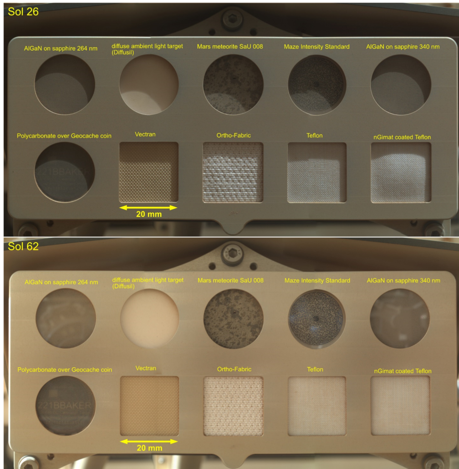
Fig. 5 WATSON image mosaics of the SCT acquired on Sol 26 (top) and 62 (bottom). The Sol 26 mosaic was illuminated by the sun from the top right; the Sol 62 mosaic was acquired with the SCT in full shadow. Both are mosaics of 3 WATSON images acquired from about 12 cm distance (about 51.0 \pm 2.5 \mu\text{m}/\text{pixel} )
