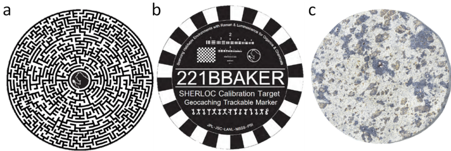
Fig. 3 Images of the three primary public outreach targets: a ) the intensity maze target, b ) the geocache coin and c ) the SaU 008 martian meteorite. Of note in b ) the checkerboard tiles are 0.025 \times 0.025 mm and the dancing man figures consist of 100 micron-wide lines
