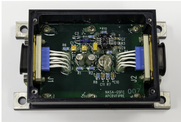
Fig. 23 Photograph of the cylinder pre-amp box with its circuit board visible which was at the base of the booms that accepted the cylindrical sensor input
