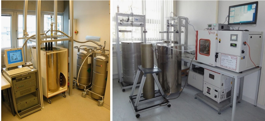
Fig. 12 Pictures of the calibration set-up at IWF (left) and at Magson GmbH (right); The IWF facility enables calibration of offsets, noise, linearity and transfer function for sensors over a temperature range between -150\text{ }^{\circ}\text{C} and 200\text{ }^{\circ}\text{C} in a low-field environment. The facility consists of a temperature controlled Dewar vessel within a three-layer magnetic shielding and a stimulus coil. At Magson, the magnetic field sensors and the electronics box were placed in three different shielding cans and a temperature control chamber, respectively, for drift measurements at different electronics temperatures
