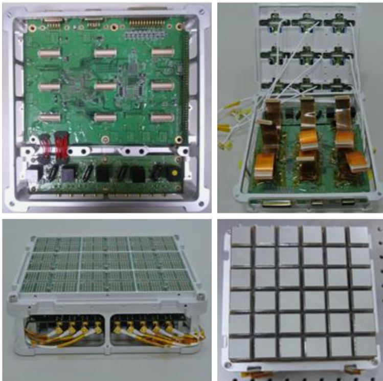
Fig. 3 UBAT detector assembly. Top left : Digital board and high voltage board. Top right : UBAT detector top and bottom parts. 9 analog boards are resident and every analog board is connected to the digital board via FPCB and to the high voltage board using high voltage cables. Bottom left : Assembly view after connection of digital board, analog boards, and high voltage board onto the UBAT detector structure. Bottom right : Integration of 36 MAPMTs and 36 YSO Scintillation crystal arrays onto the analog boards. MAPMTs are inserted directly onto analog boards using holetite
