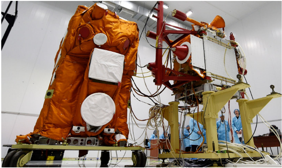
Fig. 4 Integration of Lomonosov payloads (left, orange) to the spacecraft (right, white). The UBAT is shown as a white rectangle at the center of the payloads, and the SMT is shown as a white circle at the bottom of the payloads. (Courtesy of Roscosmos)
