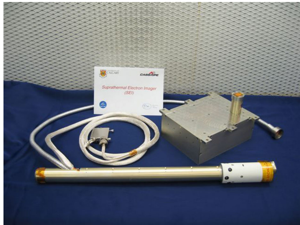
Fig. 2 The e-POP SEI sensor and boom assembly, electrical and fiber optic cables, and electronics unit (EU). Photo: E. Peter King
