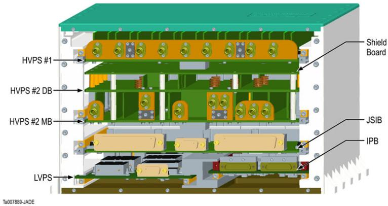
**Fig. 29** The JADE Electronics Box
