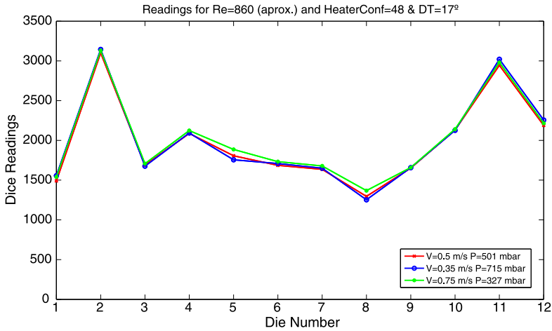
Fig. 21 Dice readings at identical Reynolds number, but with different combinations of pressure and speed. As the temperature of all tests is the same, the conduction and radiation losses are identical, and therefore the injected power to each die can be compared varying only pressure and speed. These results correspond to tests at Yaw = 0° and Pitch = 0°
