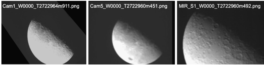
Fig. 20 Single unprocessed images taken (left to right) VIS/Cam1, NIR1/Cam5 (1.4–1.7 \mu\text{m} ) and MIR1/MIR_S1 (6–10 \mu\text{m} ) during lunar swingby (DOY09-174) target 2 measurements and rotated to align to same view. The FOVs are 30.1^\circ \times 22.8^\circ , 28.7^\circ \times 21.7^\circ , and 15.0^\circ \times 11.0^\circ , respectively. LCROSS was \sim 8,800 km altitude from the Moon at this point in the swingby. NIR1 is slightly out of focus, a known issue prior to launch
