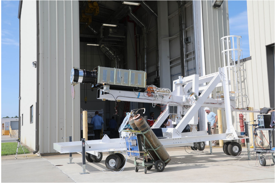
Figure 12 The coronagraph integrated to the gondola and WASP system (the telescope beam, gimbals, Sun sensor, and the associated computer) at WFF. The doghouse is placed over the coronagraph. The gondola was rolled outside the hangar for a Sun-pointing test. The nitrogen gas tanks in the foreground are for pushing the purge gas through the coronagraph system to keep the optics elements clean. The gondola is attached to tie ropes that connect to the rotator and then to the balloon.
