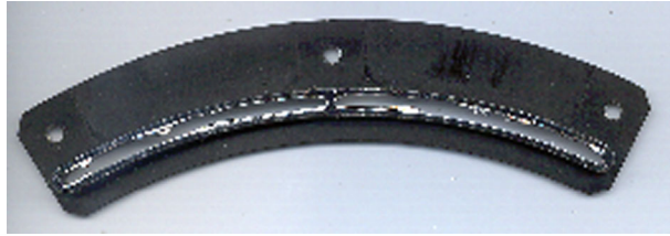
Figure 5 SXT entrance filter frame. The filter membrane itself has been destroyed in testing, showing the catastrophic degradation typical of the failure of thin films of this type.
