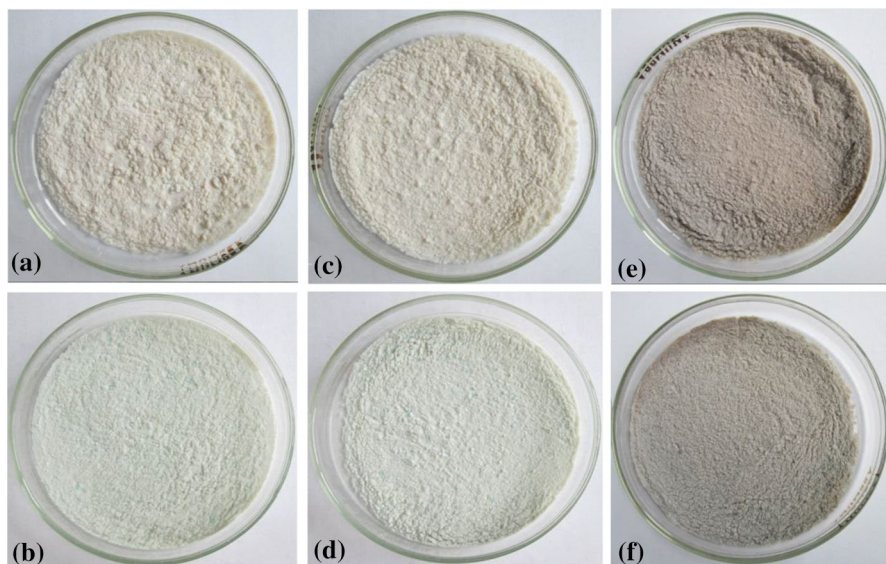
Fig. 9 Images of samples: 02Ag-F (upper row) and 02Ag02Cu-F (bottom row) before irradiation (a, b), after under UV light for 60 min (c, d), and after sunlight exposure for 10 days (e, f)
