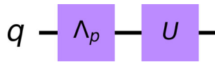
Fig. 10 Incoherent noise model. The gate \Lambda is introduced to the channel with probability p and the identity gate I with probability 1 - p
