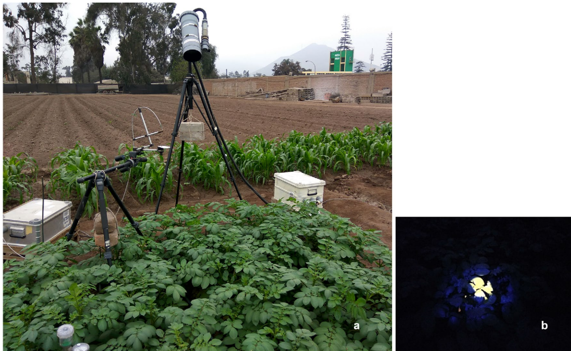
Fig. 5 a Measurement configuration of Ledflex and Spectroflex over the vegetation cover of a potato plot. b Photograph of the plot acquired at night showing the effective area measured by both instru-
