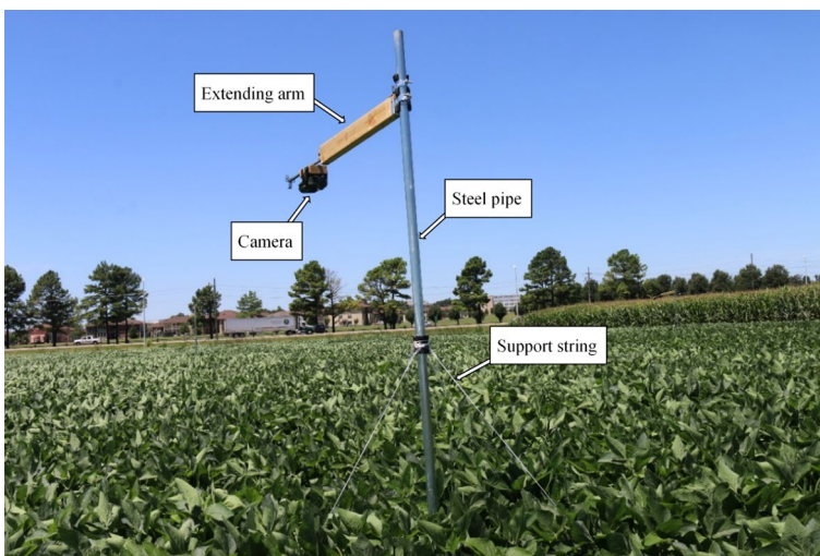
Fig. 2 One of the game and trail time-lapse cameras installed in the soybean field
